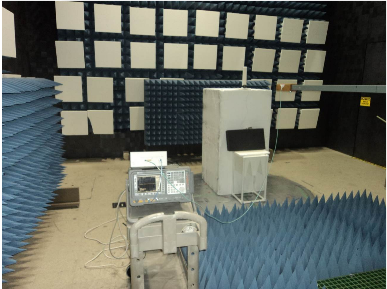
Figure 5: Typical Radiated Emissions – 18 GHz to 24 GHz shown, Front view
