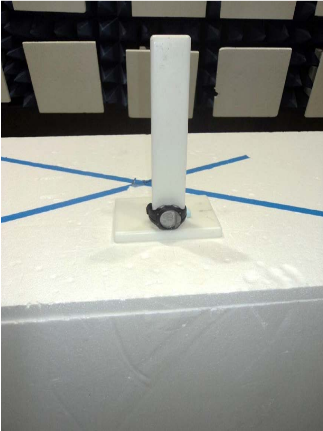
Figure 10: Radiated Emissions Test Setup – Receive only (Unintentional Radiator)
