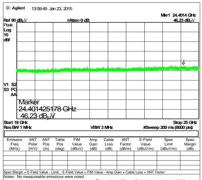
No correction factors were used for the above graph. The number of Sweep Points was increased to 8000.
