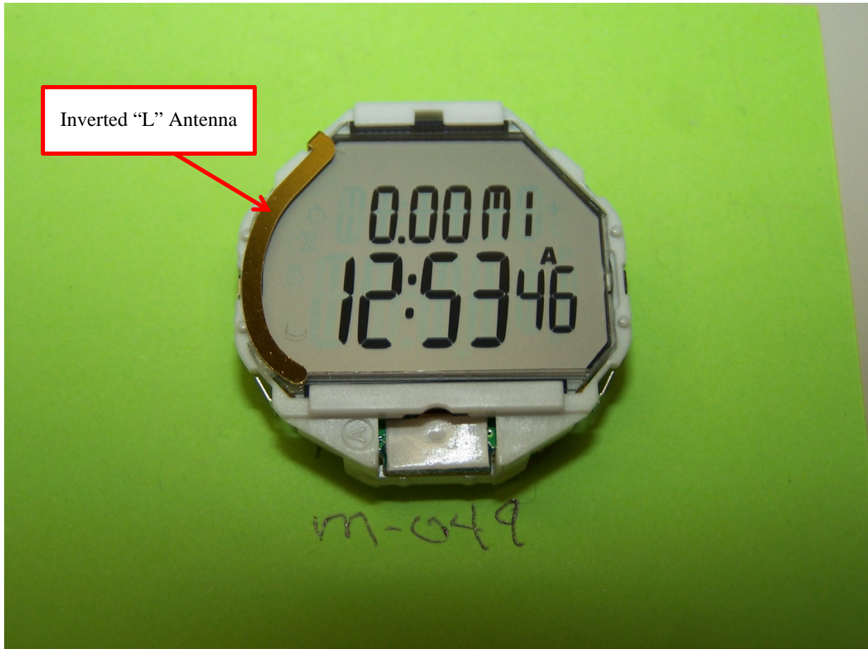
Figure 2: Front View of watch module showing the Display and BLE antenna.
