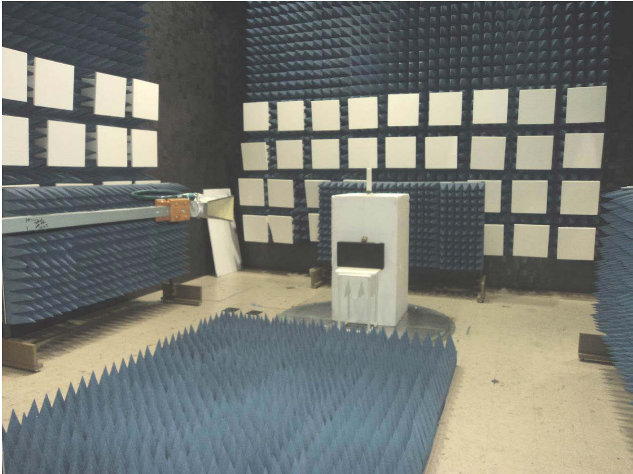
Figure 3: Typical Radiated Emissions – 1 GHz to 18 GHz shown, Front view
