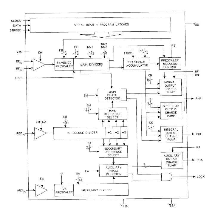
Figure 1: DL-3412 SYNTHESIZER INTEGRATED CIRCUIT (U811)
