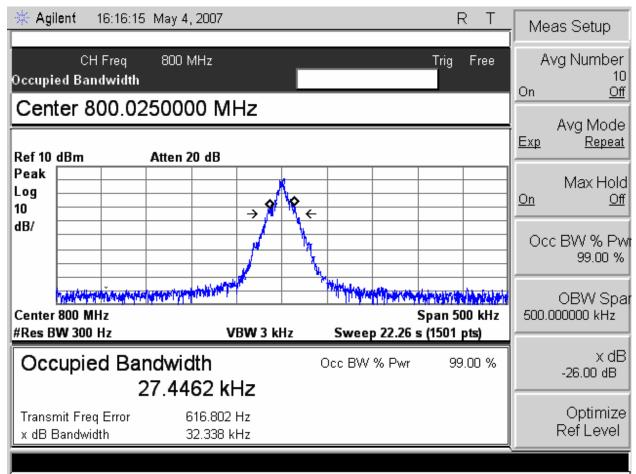
A OCBW plot for all three subsets of modulation (16FSK, 8FSK and 4FSK) is provided below. For this capture the RBW was set to 1kHz to allow faster sweeps and the peak hold mode capture was ran over more traces
