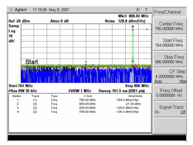
Notch filter 1 cavity from . Center frequency 800.025 attenuation 34.8dB (not on the plot display). Marker 1-794.0MHz @ -2.6dB, Marker 2 – 776.0MHz @ -0.4dB, Marker 3 – 799.425MHz @ -19.5dB, 4.0MHz/division span
