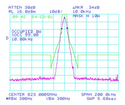
Note: For frequencies spaced more than 25kHz from the central frequency the attenuation should read 59dBc at 40W. The plot above reads 53dBc as indicated in the description of the set-up.
