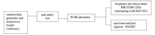
NAME OF TEST: Transmitter Occupied Bandwidth
