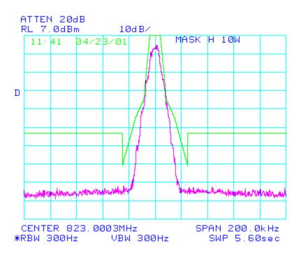
Note: For frequencies spaced more than 25kHz from the central frequency the attenuation should read 50dBc at 5W. The plot above reads 53dBc as indicated in the description of the set-up.
