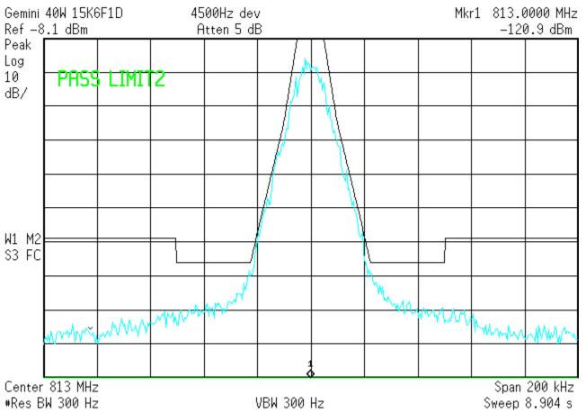
NAME OF TEST: Transmitter Occupied Bandwidth
