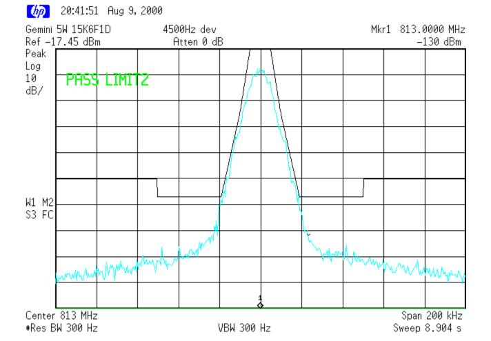
MASK: G, 15K6F1D, 40W SPECTRUM FOR EMISSION 15K6F1D **OUTPUT POWER: 40 Watts** 12800 bauds 4 level FSK PEAK DEVIATION = 4500 Hz
