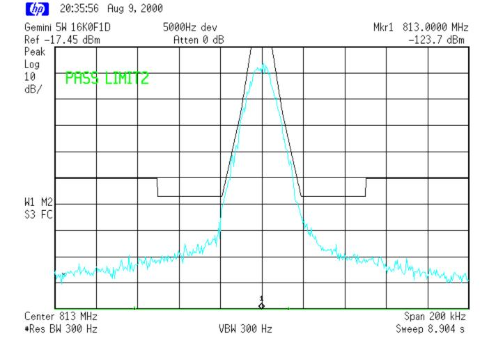
MASK: G, 16K0F1D, 40W SPECTRUM FOR EMISSION 16K0F1D **OUTPUT POWER: 40 Watts** 9600 bauds, 4 level FSK PEAK DEVIATION = 5000 Hz SPAN = 200 kHz
