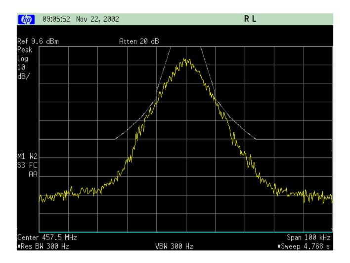
NAME OF TEST: Transmitter Occupied Bandwidth
