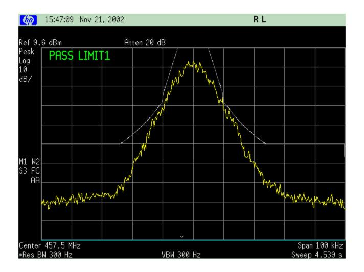
NAME OF TEST: Transmitter Occupied Bandwidth
