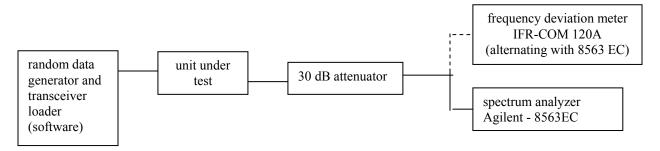
NAME OF TEST: Transmitter Occupied Bandwidth
