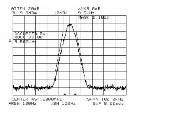
Note: For frequencies spaced more than 12.5kHz from the central frequency the required attenuation is 60dBc at 10W.
