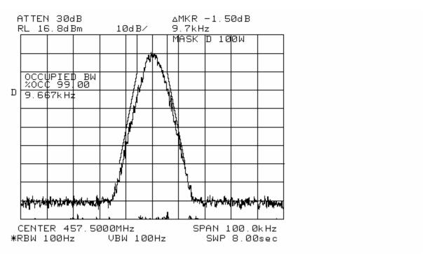
Note: For frequencies spaced more than 12.5kHz from the central frequency the required attenuation is 67dBc at 50W.
