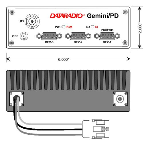
Figure 5 - Front and rear panels
