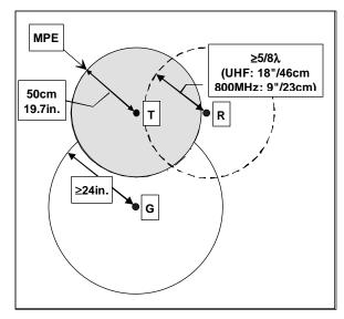
Figure 4 - Antenna spacing
