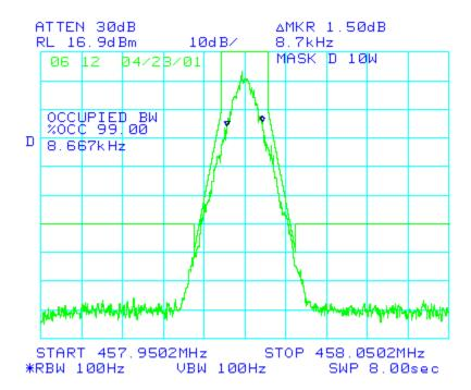
Note: For frequencies spaced more than 12.5kHz from the central frequency the attenuation should read 67dBc at 50W. The plot above reads 60dBc as indicated in the description of the set-up.
