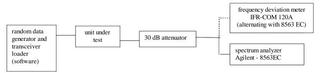
NAME OF TEST: Transmitter Occupied Bandwidth
