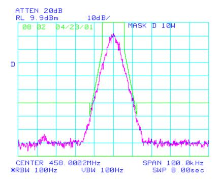
MASK: D, 8K67F1D, 50W SPECTRUM FOR EMISSION **8K67F1D** OUTPUT POWER: 50 Watts 7200 bauds, 4 level FSK PEAK DEVIATION = 2350 Hz
