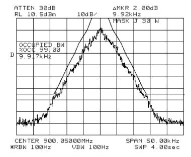
GEMINI Modem at 9600 bps DGMSK In Support of Emission Designator **10K2F1D**
