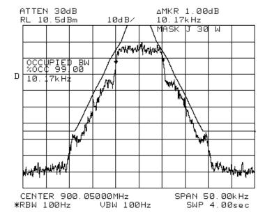
GEMINI Modem at 8000Bps DGMSK In Support of Emission Designator **8K75F1D**
