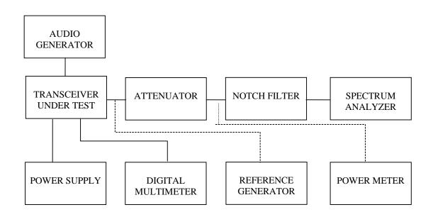
NAME OF TEST: Transmitter Spurious and Harmonic Outputs
