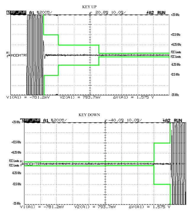
TRANSIENT FREQUENCY RESPONSE UHF 438-512MHz Exciter: Unmodulated 400 mWatts
