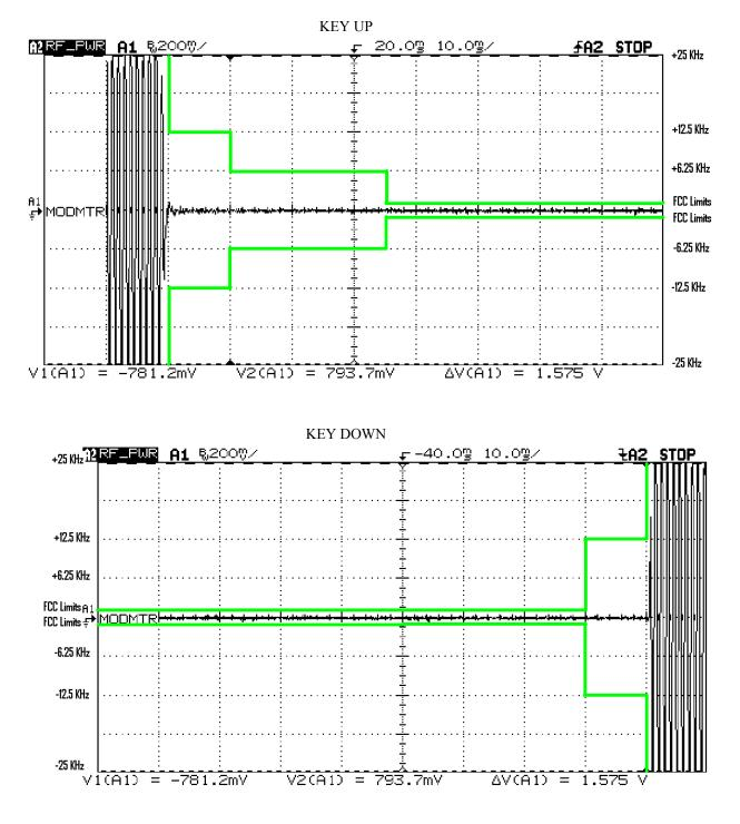
TRANSIENT FREQUENCY RESPONSE UHF LOW Exciter : Unmodulated 400 mWatts
