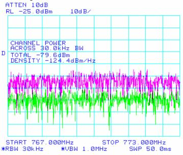
All the power channel read was below -78.5dBm/30kHz, after the correction of the 2.1dB inserted by the notch filter the absolute channel coupled power was found lower than -76.4dBm The value required for maximum absolute ACCP =-75dBm/30kHz bandwidth. >-76.4dBm The value required for maximum relative ACCP = -100dBc >120dBc Test results 1W (power control at maximum power reduction 90.534(b)(4)
