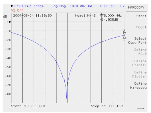
Two cavities notch (1000kHz frequency offset and in the receive band) 39MHz sweep, 3.9MHz/div Attenuation between -45dB <a<-30dB for frequency offset 600kHz to 1MHz ▶1:S21 Fwd Trans Log Mag 10.0 dB/ Ref 0.00 dB C? HARDCOPY ⊳2:Off 2004-06-04 11:19:00 Meas1:Mkr2 806.000 MHz Start dB -1.25\$dB 1: 🕨 Abort -10Select -20 Copy Port -30 Define PCL5 -40 Define Printer -50 Define -60 Plotter Define -70 Hardcopy -80 Start 767.000 MHz Stop 806.000 MHz
