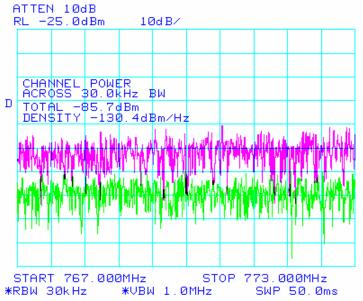
All the power channel read was below -82.3dBm/30kHz, after the correction of the 2.1dB inserted by the notch filter the absolute channel coupled power was found lower than -80.2dBm The value required for maximum absolute ACCP =-75dBm/30kHz bandwidth. >-80.2dBm The value required for maximum relative ACCP = -100dBc >120dBc General settings of the instrument
