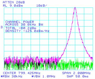
All the power channel read was below -75dBm/30kHz, after the correction of the 17dB (worst case) inserted by the notch filter the absolute channel coupled power was found lower than -58dBm The value required for maximum absolute ACCP = -45dBm/30kHz bandwidth. >-58dBm The value required for maximum relative ACCP = -60dBc >103dBc
