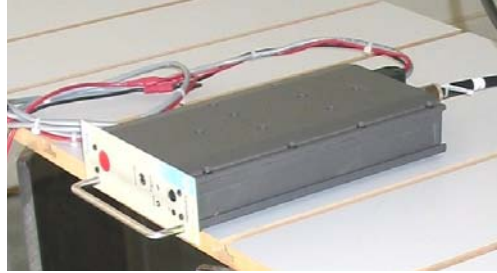
DataRadio T881-10 700 MHz band base station tested for radiated spurious emissions
