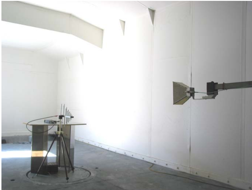
Dataradio T881-10 700 MHz band base station tested for Spurious Emissions from Transmitter Frequency Range: 30 MHz – 18 GHz
