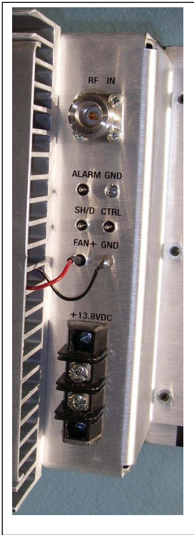
Figure 5 - Power Amplifier's DC Power and RF Connectors on Rear Side
