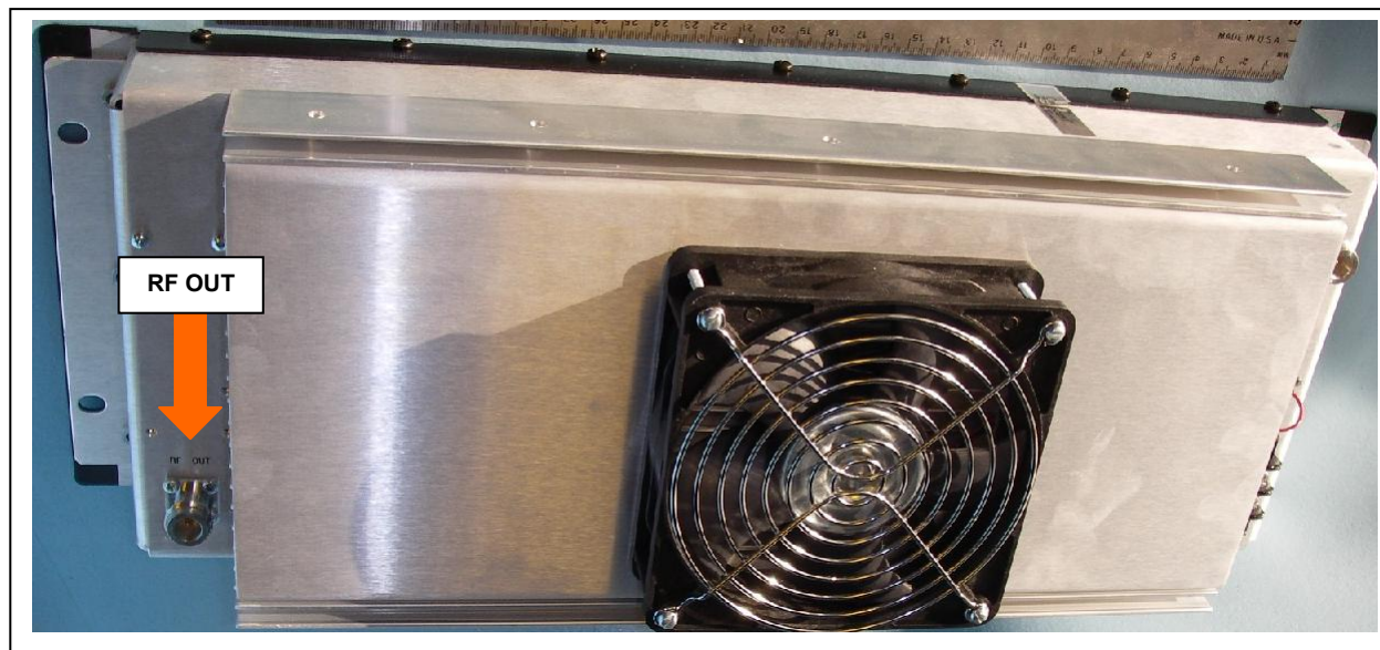
Figure 3 – Crescend Technologies 70W Power Amplifier – Rear View Underlining the RF Out Connector
