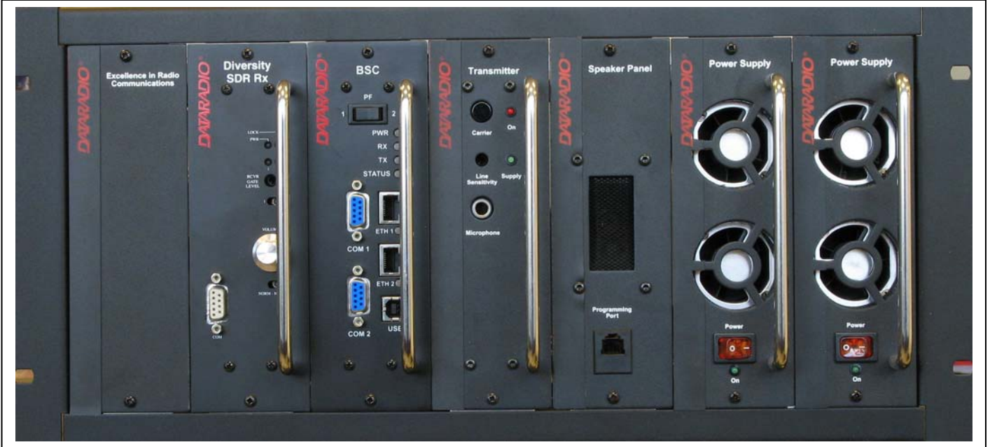
Figure 1 - Typical rack-mount multi-modules "Radio Assembly"
