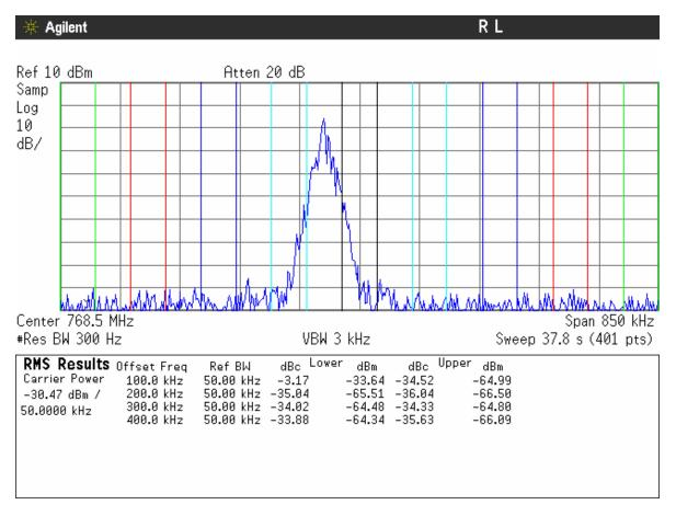
UUT in right channel (+50kHz) of the 150kHz 3-contiguous 50 kHz channels .
