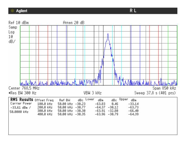
50 kHz channel (non-aggregated) adjacent channel coupled power. Test channel, frequency 768.500 MHz. All power readings on 50kHz channel
