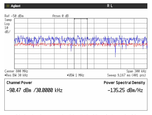
Across all the channel, maximum power read was below -80.0 dBm/30 kHz, after the correction of the 17.8dB inserted by the set-up (notch filter plus attenuators) the absolute channel coupled power was found lower than -62.2 dBm
