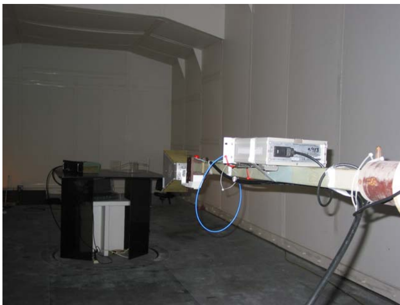
DataRadio EOTBDP3-AMP Amplifier tested for Spurious Emissions from Transmitter Frequency Range: 30 MHz – 18 GHz
