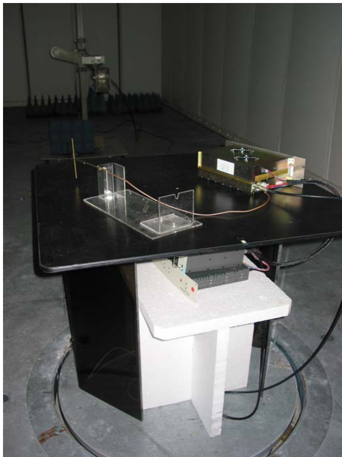
DataRadio EOTBDP3-AMP Amplifier (system configuration tested for radiated spurious emissions)
