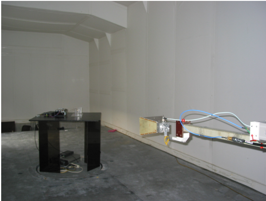
Dataradio Aethercomm 700 MHz band base station tested for Spurious Emissions from Transmitter Frequency Range: 30 MHz – 18 GHz
