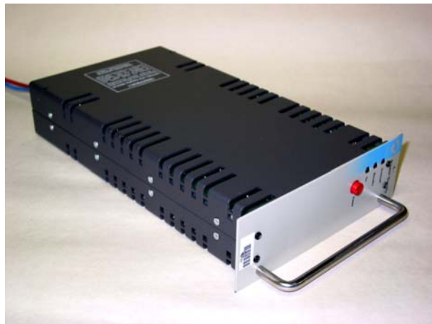
DataRadio Aethercomm 700 MHz Band Base Station (system components used in test)
