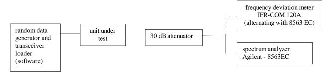
NAME OF TEST: Transmitter Occupied Bandwidth
