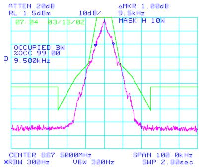
SPECTRUM FOR EMISSION 9K50F1D **OUTPUT POWER: 1 Watt** 19200bps, 9600 bauds, 4 level FSK PEAK DEVIATION = 2100 Hz SPAN = 100 kHz
