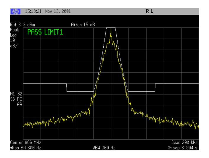
MASK: G, 1W OUTPUT POWER: 1 Watt 16000 bauds, 4 level FSK PEAK DEVIATION = 3630 Hz SPAN = 200 kHz
