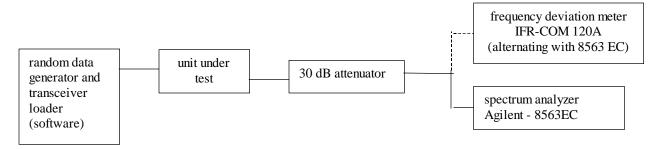
NAME OF TEST: Transmitter Occupied Bandwidth
