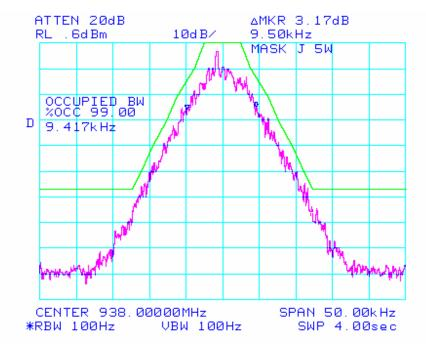
NAME OF TEST: Transmitter Occupied Bandwidth
