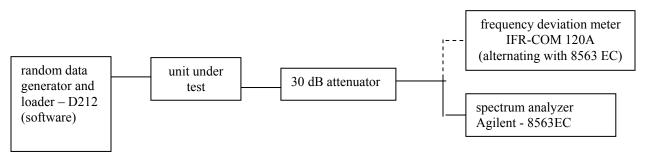
NAME OF TEST: Transmitter Occupied Bandwidth
