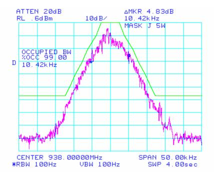
NAME OF TEST: Transmitter Occupied Bandwidth
