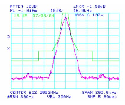
156-90000-780 Dataradio<sup>©</sup> FCC submission MASK: 14400baud, 4.2kHz dev, 100 W
