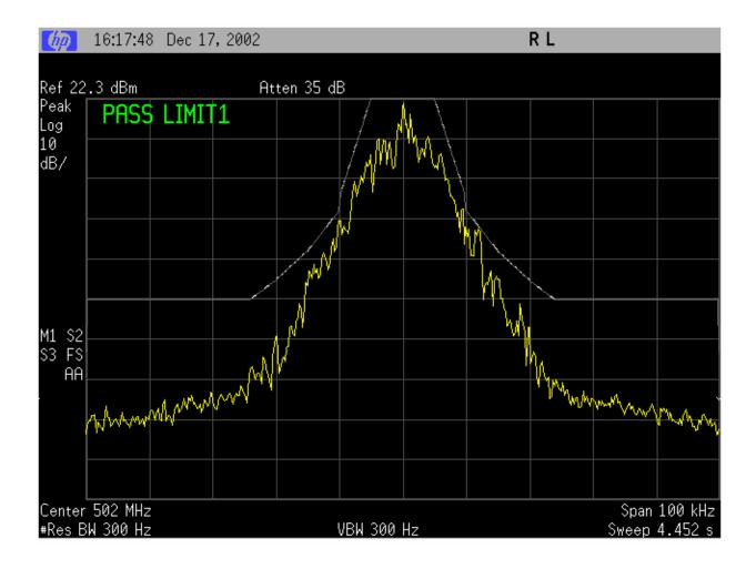
MASK: C, 16K7F1D, 20 W SPECTRUM FOR EMISSION 16K7F1D OUTPUT POWER: 20 Watts 48000 bps, 8 level FSK PEAK DEVIATION = 5030 Hz SPAN = 100 kHz
