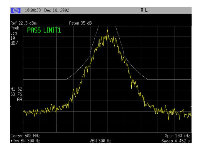
MASK: C, 14K9F1D, 20 W SPECTRUM FOR EMISSION **14K9F1D** OUTPUT POWER: 20 Watts 43200 bps, 8 level FSK PEAK DEVIATION = 4820 Hz SPAN = 100 kHz
