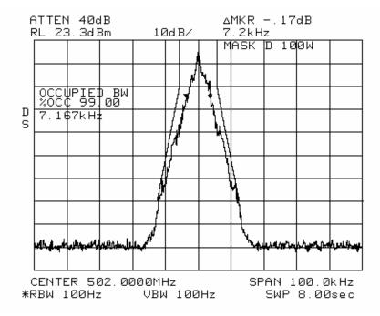
MASK: D, 7K17F1D, 20 W SPECTRUM FOR EMISSION **7K17F1D** OUTPUT POWER: 20 Watts 16000 bps, 4 level FSK PEAK DEVIATION = 1840 Hz SPAN = 100 KHz
