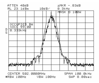
MASK: D, 8K33F1D, 20 W SPECTRUM FOR EMISSION **8K33F1D** OUTPUT POWER: 20 Watts 21600 bps, 8 level FSK PEAK DEVIATION = 2920 Hz SPAN = 100 KHz
