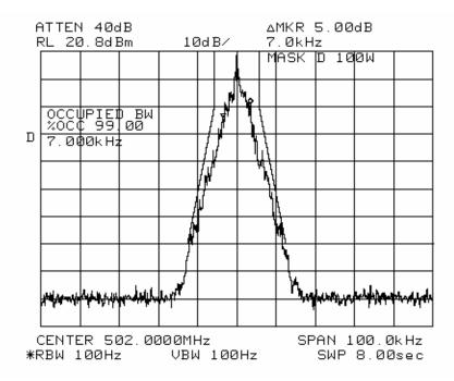
NAME OF TEST: Transmitter Occupied Bandwidth
