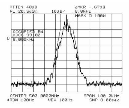
NAME OF TEST: Transmitter Occupied Bandwidth
