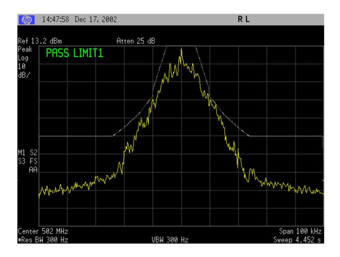
MASK: C, 16K7F1D, 100 W SPECTRUM FOR EMISSION **16K7F1D** OUTPUT POWER: 100 Watts 48000 bps, 8 level FSK PEAK DEVIATION = 5030 Hz
