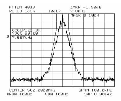
MASK: D, 8K00F1D, 20 W SPECTRUM FOR EMISSION **8K00F1D** OUTPUT POWER: 20 Watts 24000 bps, 8 level FSK PEAK DEVIATION = 2590 Hz SPAN = 100 KHz
