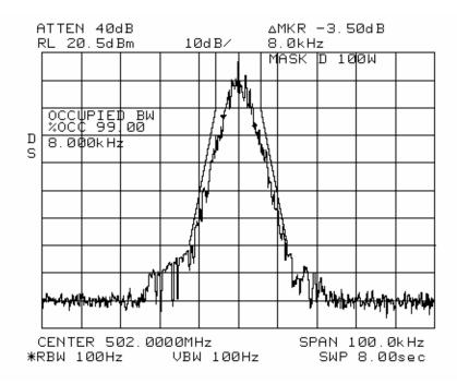
NAME OF TEST: Transmitter Occupied Bandwidth
