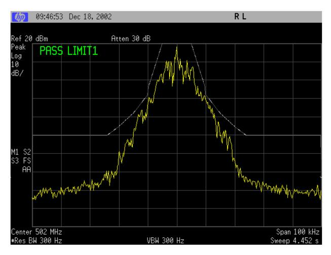
NAME OF TEST: Transmitter Occupied Bandwidth
