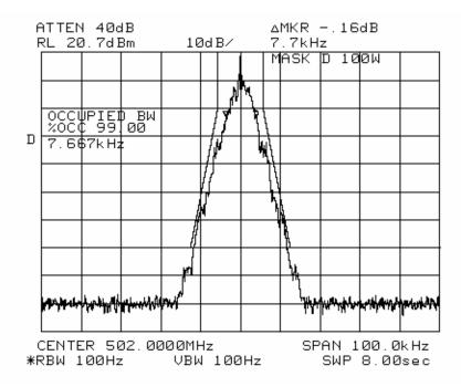
NAME OF TEST: Transmitter Occupied Bandwidth
