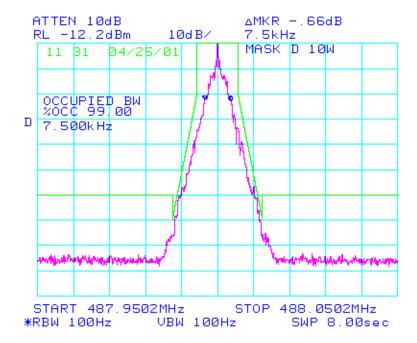
Note: For frequencies spaced more than 12.5kHz from the central frequency the required attenuation should read 70dBc at 100W. The plot above reads 60dBc as indicated in the description of the set-up. The measured emission bandwidth is within the actual requirement.
