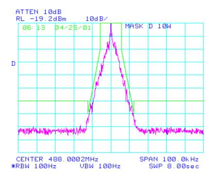
Note: For frequencies spaced more than 12.5kHz from the central frequency the required attenuation should read 63dBc at 20W. The plot above reads 60dBc as indicated in the description of the set-up. The measured emission bandwidth is within the actual requirement.
