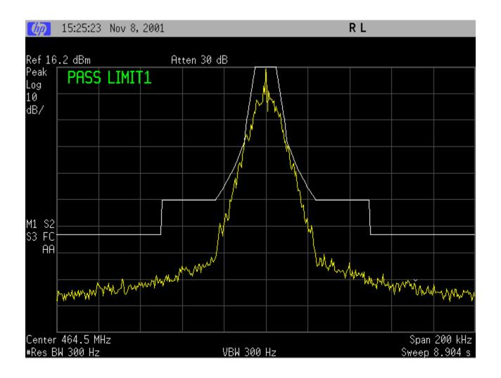
MASK: C, 16K5F1D, 20W SPECTRUM FOR EMISSION **16K5F1D** OUTPUT POWER: 20 Watts 16000 bauds, 4 level FSK PEAK DEVIATION = 4340 Hz SPAN = 200 kHz
