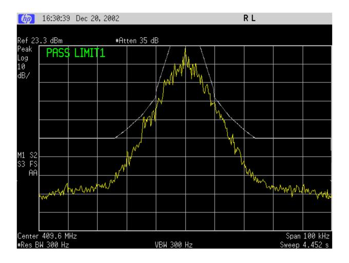
MASK: C, 14K9F1D, 20 W SPECTRUM FOR EMISSION **14K9F1D** OUTPUT POWER: 20 Watts 43200 bps, 8 level FSK PEAK DEVIATION = 4550 Hz SPAN = 100 kHz
