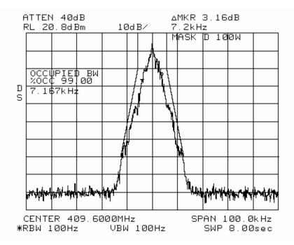
NAME OF TEST: Transmitter Occupied Bandwidth
