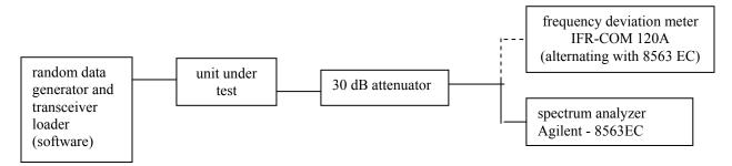
NAME OF TEST: Transmitter Occupied Bandwidth
