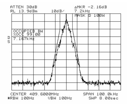
MASK: D, 7K17F1D, 100 W SPECTRUM FOR EMISSION **7K67F1D** OUTPUT POWER: 100 Watts
