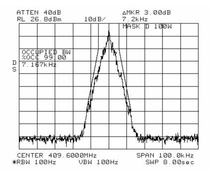
MASK: D, 7K17F1D, 20 W SPECTRUM FOR EMISSION **7K17F1D** OUTPUT POWER: 20 Watts 16000 bps, 4 level FSK PEAK DEVIATION = 1730 Hz SPAN = 100 KHz
