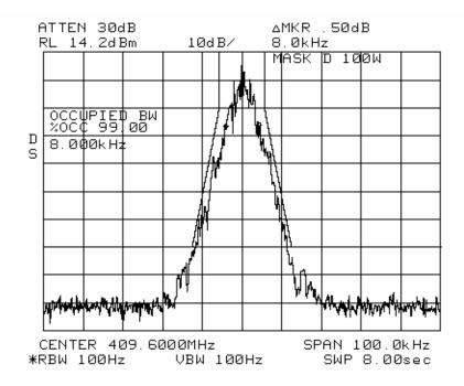
MASK: D, 8K00F1D, 100 W SPECTRUM FOR EMISSION **8K00F1D** OUTPUT POWER: 100 Watts 24000 bps, 8 level FSK PEAK DEVIATION = 2520 Hz
