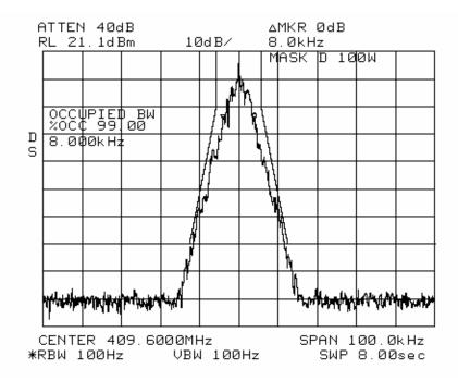
NAME OF TEST: Transmitter Occupied Bandwidth
