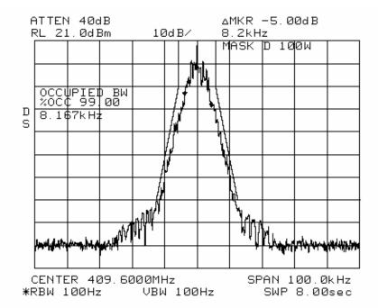
NAME OF TEST: Transmitter Occupied Bandwidth
