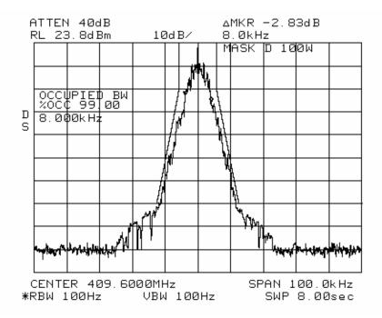
MASK: D, 8K33F1D, 20 W SPECTRUM FOR EMISSION 8K33F1D OUTPUT POWER: 20 Watts 21600 bps, 8 level FSK PEAK DEVIATION = 2840 Hz SPAN = 100 KHz
