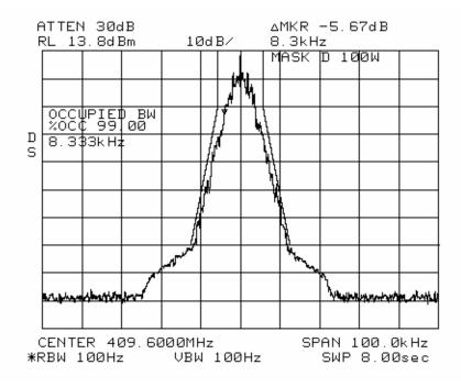
MASK: D , 8K33F1D, 100 W SPECTRUM FOR EMISSION **8K33F1D** OUTPUT POWER: 100 Watts
