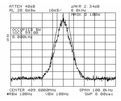
NAME OF TEST: Transmitter Occupied Bandwidth
