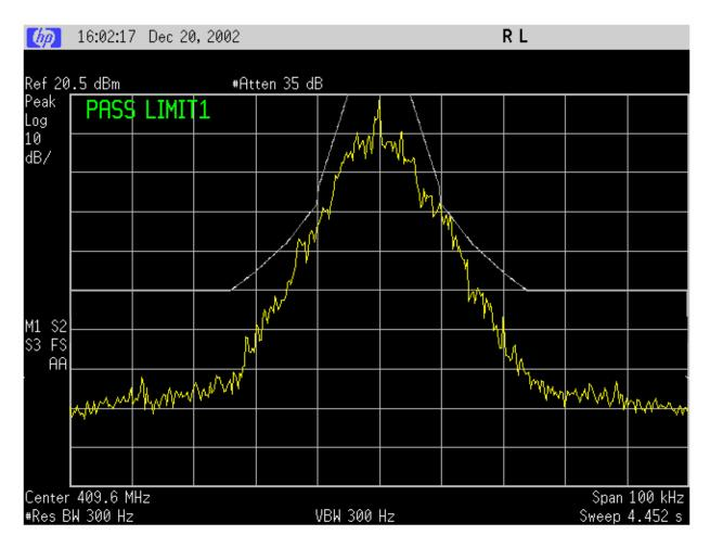
NAME OF TEST: Transmitter Occupied Bandwidth
