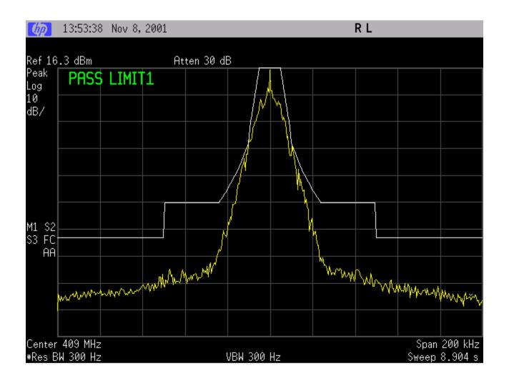
MASK: C, 16K5F1D, 20W SPECTRUM FOR EMISSION **16K5F1D** OUTPUT POWER: 20 Watts 16000 bauds, 4 level FSK PEAK DEVIATION = 4380 Hz SPAN = 200 kHz
