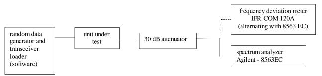
NAME OF TEST: Transmitter Occupied Bandwidth
