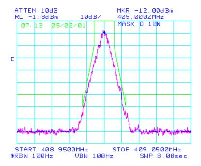
Note: For frequencies spaced more than 12.5kHz from the central frequency the required attenuation should read 50dBc at 1W. The plot above reads 60dBc as indicated in the description of the set-up. The measured emission bandwidth is within the actual requirement.
