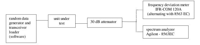
NAME OF TEST: Transmitter Occupied Bandwidth
