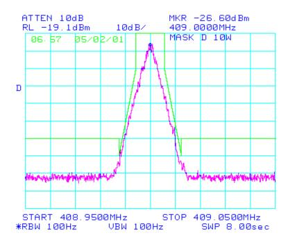
Note: For frequencies spaced more than 12.5kHz from the central frequency the required attenuation should read 63dBc at 20W. The plot above reads 60dBc as indicated in the description of the set-up. The measured emission bandwidth is within the actual requirement.
