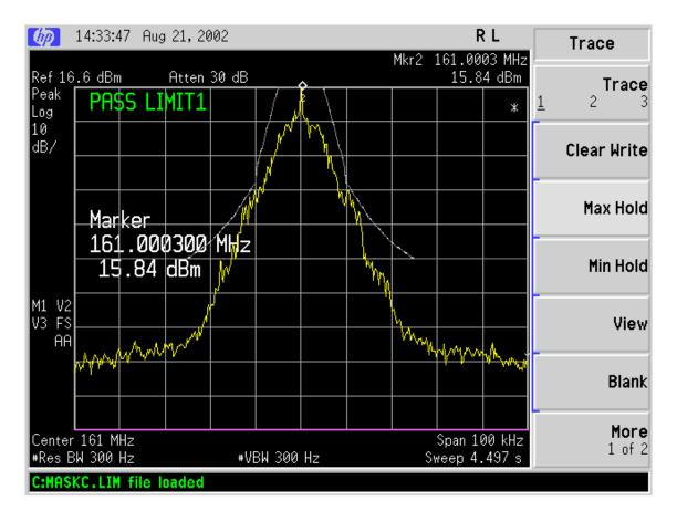
NAME OF TEST: Transmitter Occupied Bandwidth
