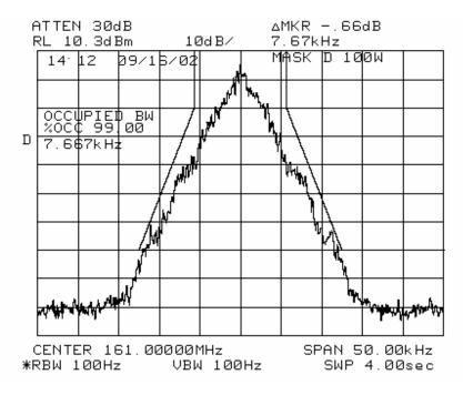
MASK: D, 7K67F1D, 100 W SPECTRUM FOR EMISSION **7K67F1D** OUTPUT POWER: 100 Watts 16000 bps, 4 level FSK PEAK DEVIATION = 1730 Hz SPAN = 50 KHz
