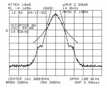
MASK: D, 14K9F1D, 20 W SPECTRUM FOR EMISSION **14K9F1D** OUTPUT POWER: 20 Watts 19200bps DGMSK PEAK DEVIATION = 4750 Hz SPAN = 100 KHz
