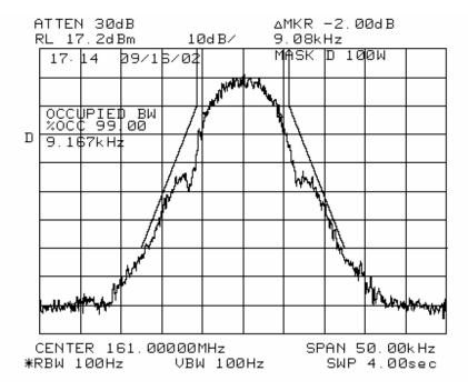
NAME OF TEST: Transmitter Occupied Bandwidth
