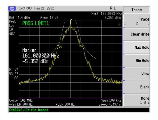
156-90000-451 Dataradio<sup>©</sup> FCC submission MASK: C, 14K7F1D, 20 W SPECTRUM FOR EMISSION 14K7F1D **OUTPUT POWER: 20 Watts** 25600 bps, 4 level FSK PEAK DEVIATION = 4120 Hz SPAN = 100 kHz
