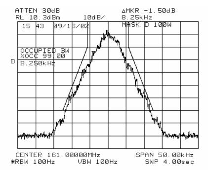
NAME OF TEST: Transmitter Occupied Bandwidth
