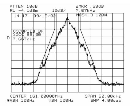
MASK: D , 7K67F1D, 20 W SPECTRUM FOR EMISSION **7K67F1D** OUTPUT POWER: 20 Watts 16000 bps, 4 level FSK PEAK DEVIATION = 1730 Hz SPAN = 50 KHz
