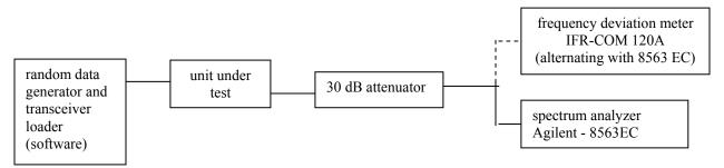
NAME OF TEST: Transmitter Occupied Bandwidth
