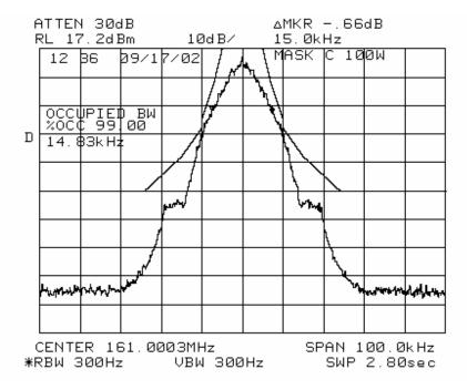
NAME OF TEST: Transmitter Occupied Bandwidth
