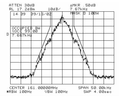
NAME OF TEST: Transmitter Occupied Bandwidth
