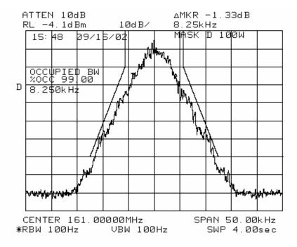
MASK: D, 8K25F1D, 20 W SPECTRUM FOR EMISSION **8K25F1D** OUTPUT POWER: 20 Watts 14400 bps, 4 level FSK PEAK DEVIATION = 2120 Hz SPAN = 50 KHz
