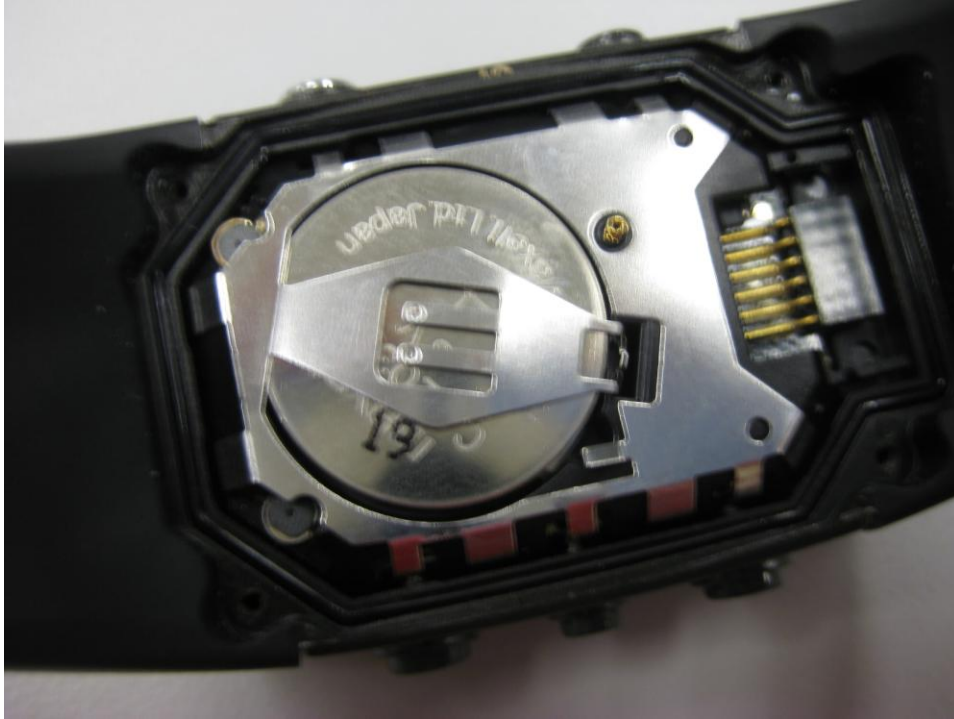
Surflink Watch bottomside assembly showing battery and battery cover
