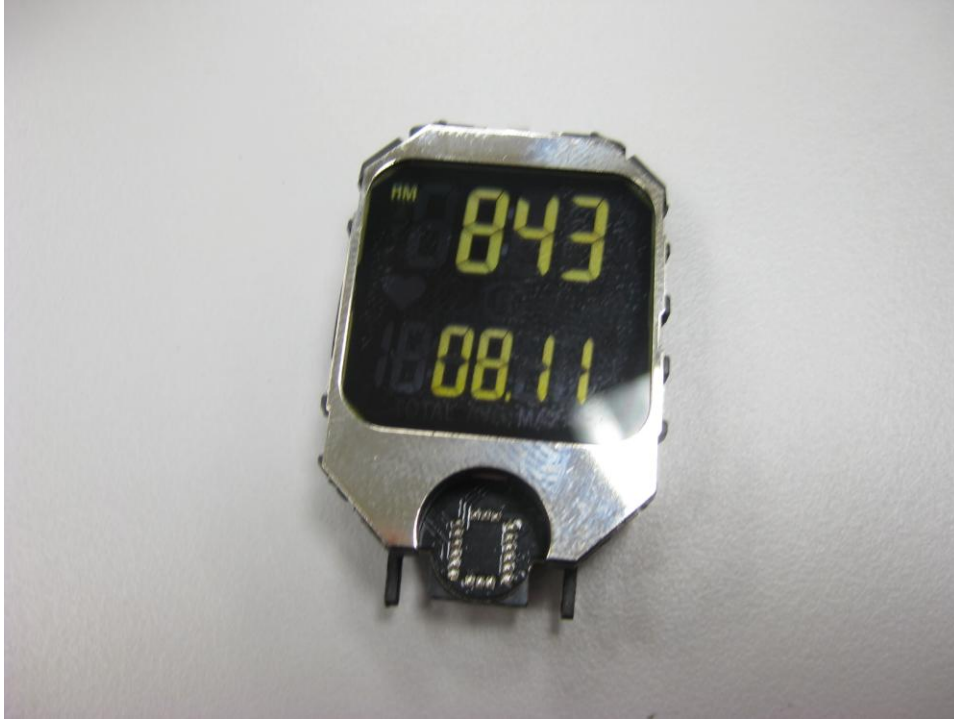
Surflink Watch topside assembly removed from housing
