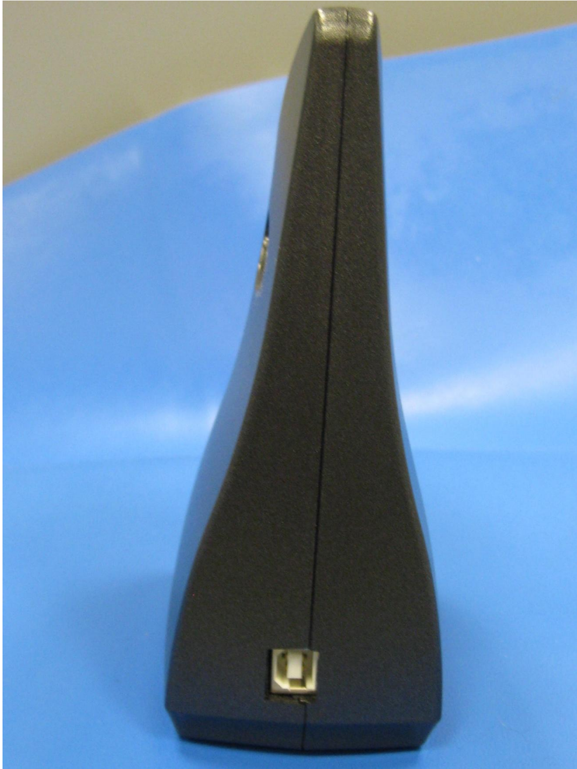
SurfLink Programmer rear view showing USB connector
