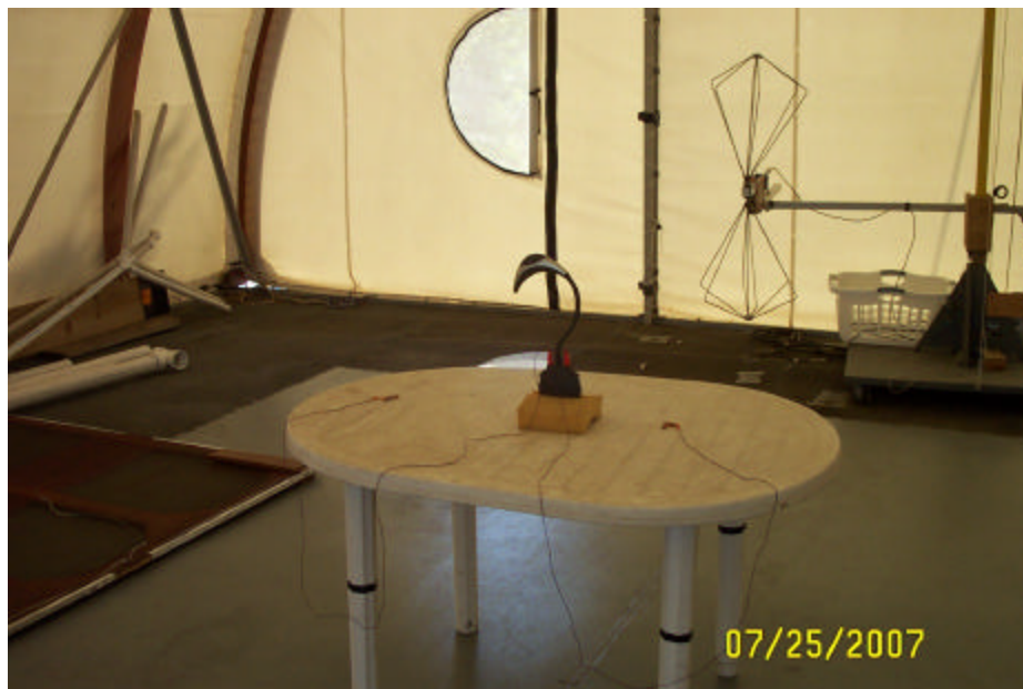
Figure 9 Radiated Emissions test configuration (Mid Frequency) FCC 15.209
