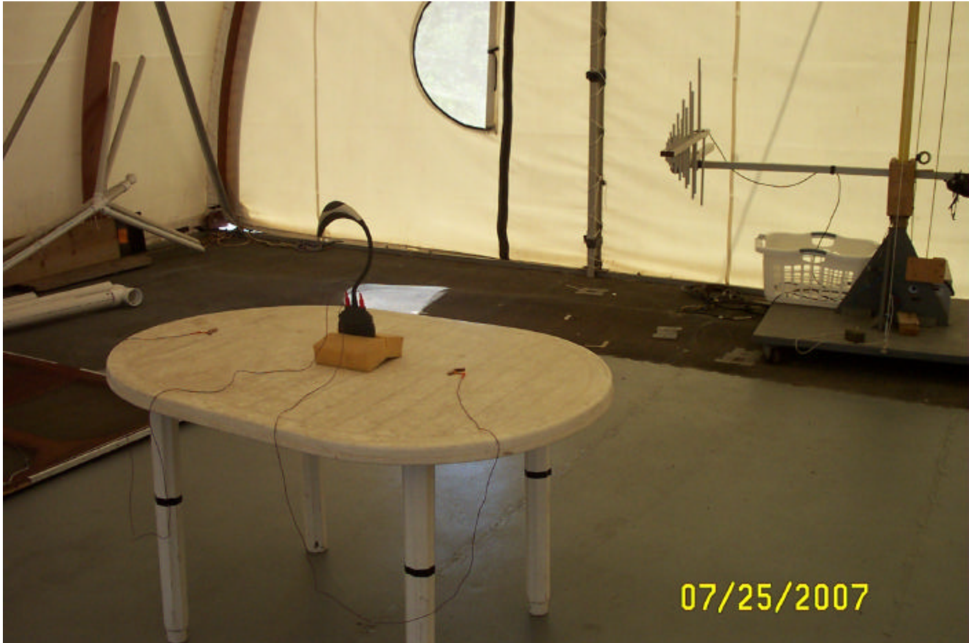
Figure 10 Radiated Emissions test configuration (High Frequency) FCC 15.209
