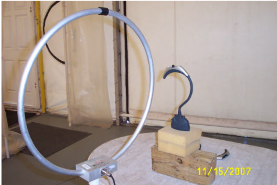
Figure 8 Radiated Emissions test configuration (Low Frequency) FCC 15.209
