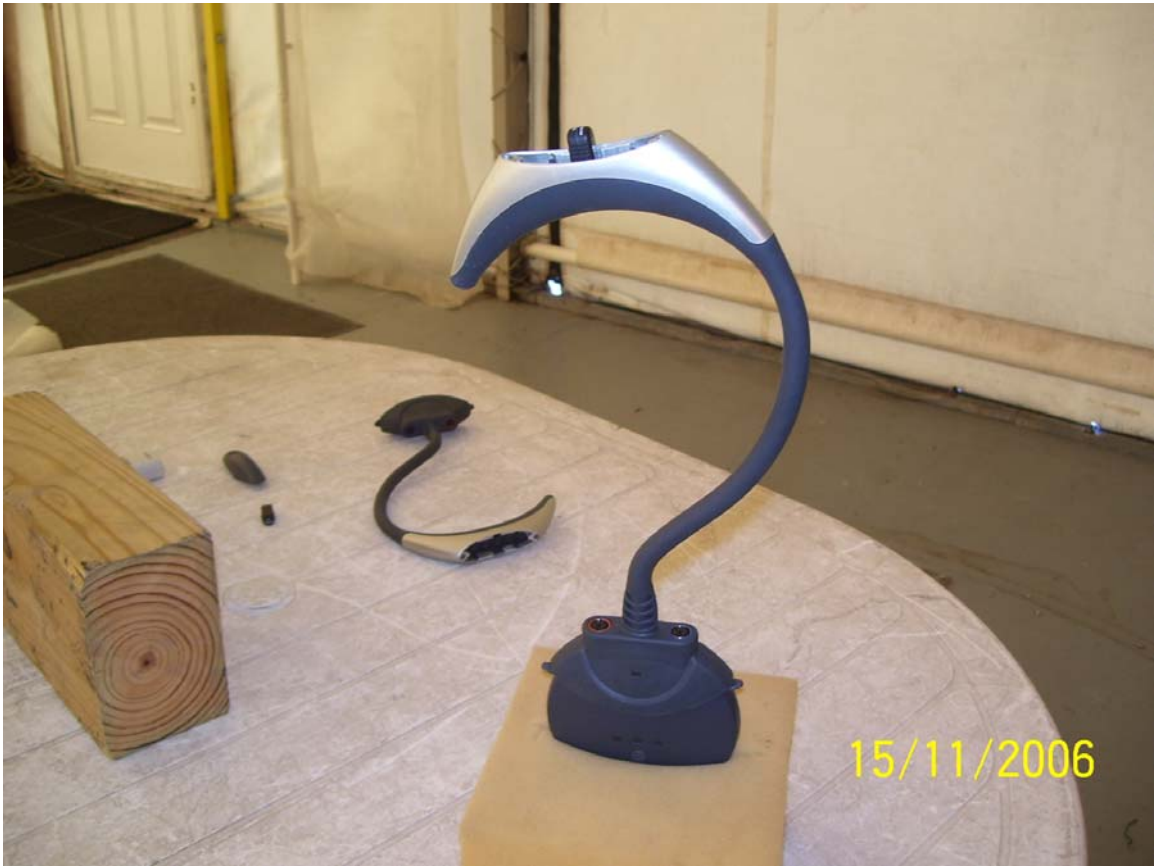
Full assembly with TM1 cover removed
