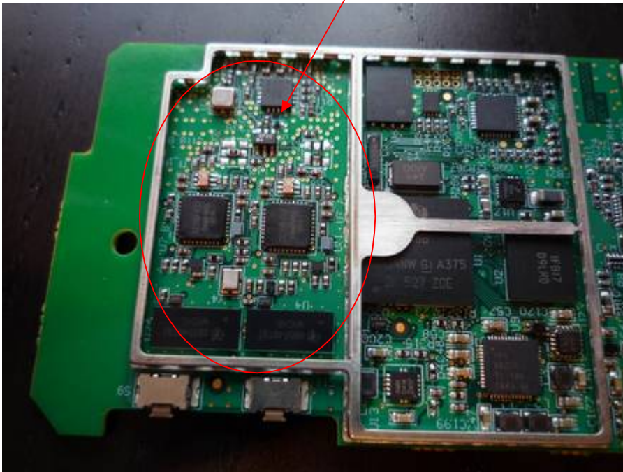
Bluetooth module (with copper tape modification)
