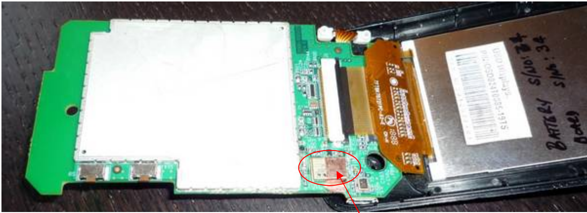
Bluetooth module (with copper tape modification)
