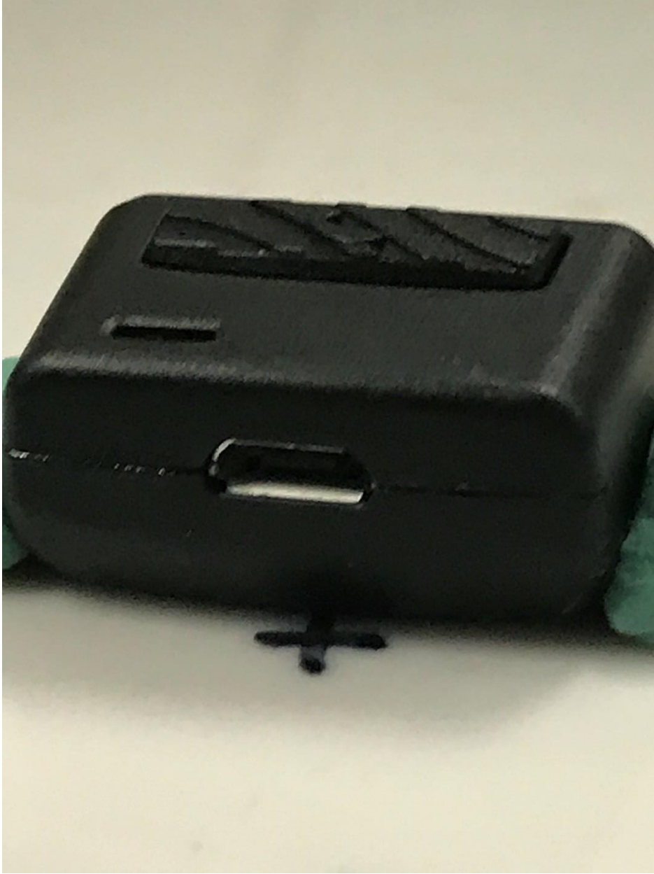
Front edge, showing female USB power input
