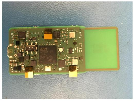
PC board front with antenna at right
