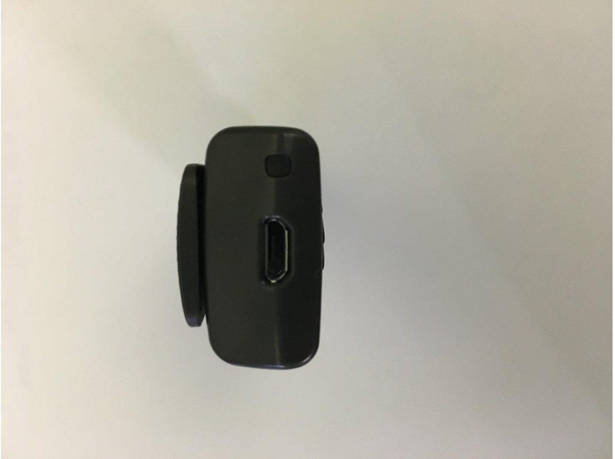
Bottom, showing USB connector and indicator LED
