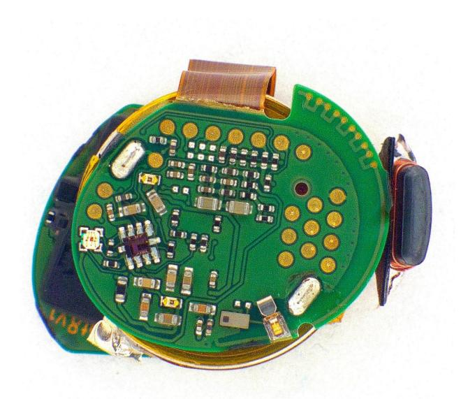
PC board bottom view (NFMI antenna on right, Bluetooth LDS antenna pickup point at 5 o'clock position)
