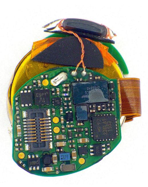
PC board top view (NFMI antenna on top)
