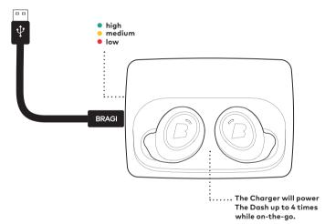
With The Dash in The Charger, connect to your computer or a power supply via USB.
