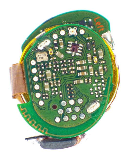
PC board bottom view (NFMI antenna on bottom)
