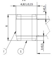
Antenna dimensions in cm are listed 4.82 cm by 6 cm overall length (4 cm coil length)
