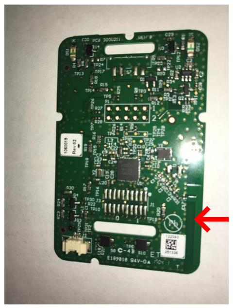
Inverted F antenna integral with PC board
