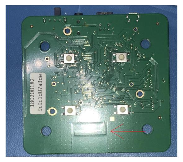
Closeup view of antenna
