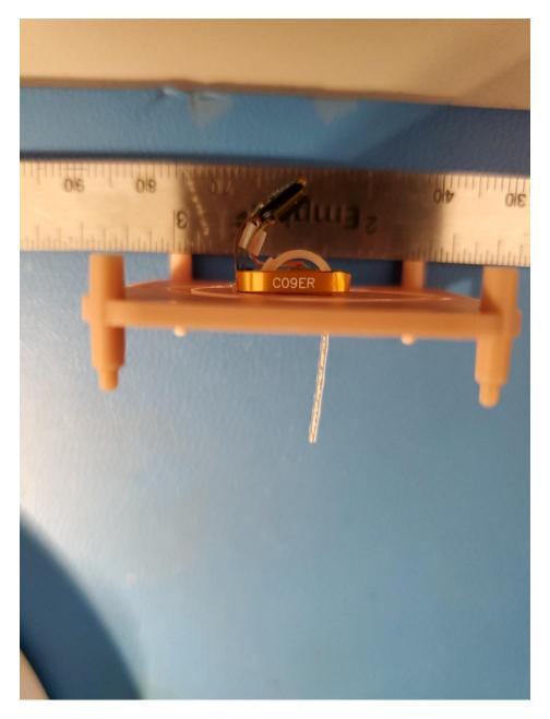
Figure 1 2.4 GHz Antenna (scale in mm)
