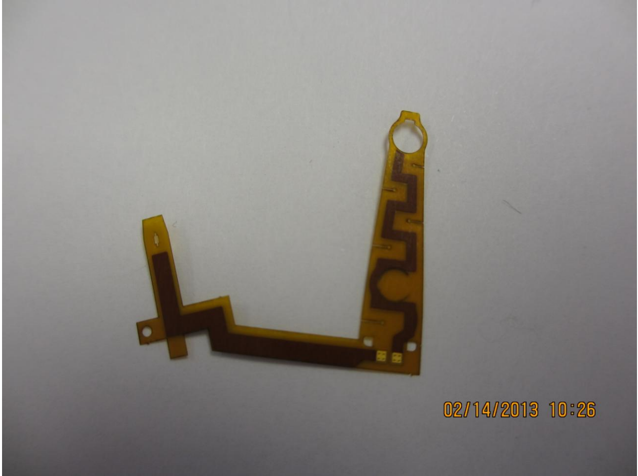
XF13 Internal Photo showing bottomside of antenna PCB
