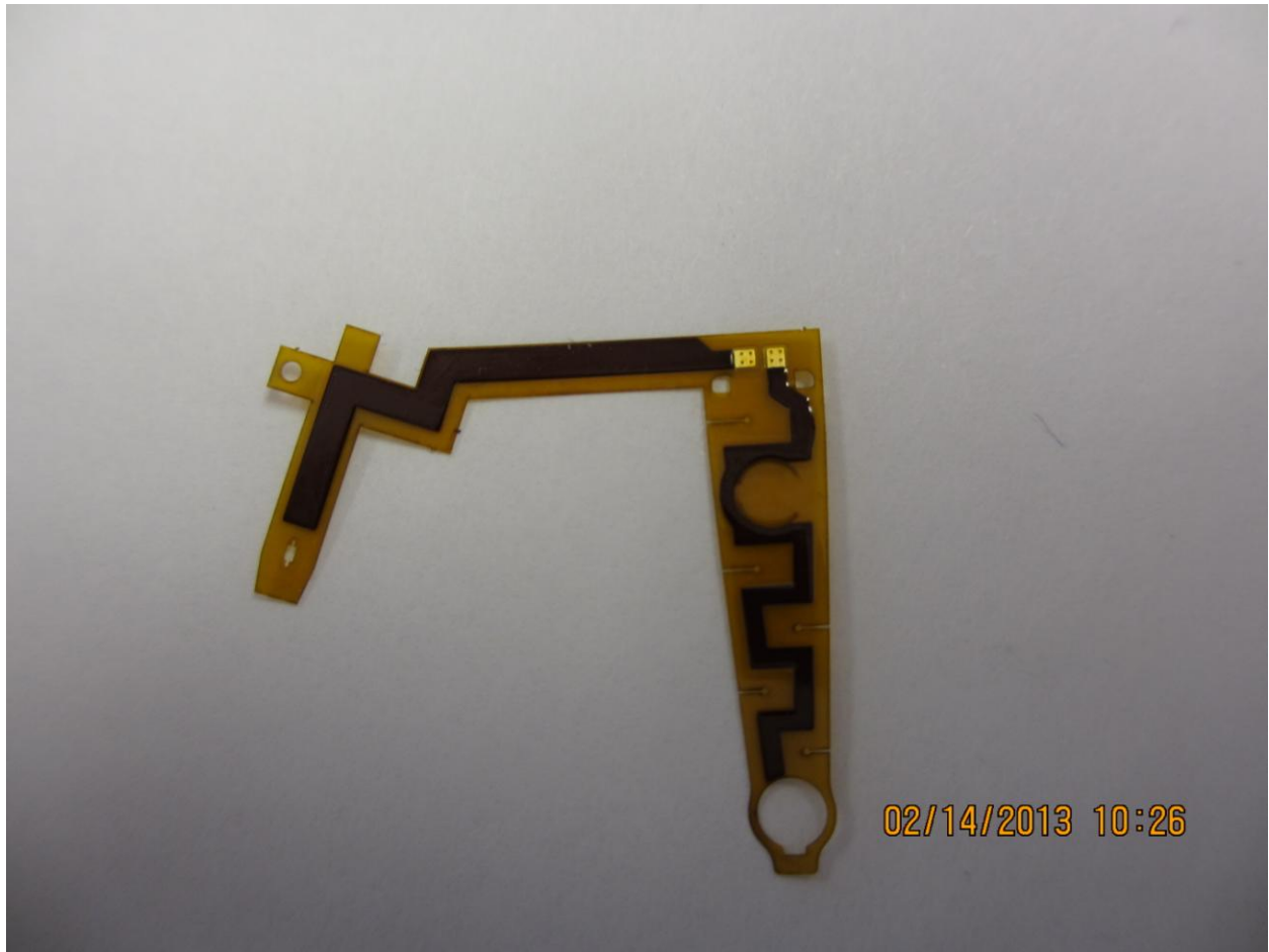
XF13 Internal Photo showing topside of antenna PCB
