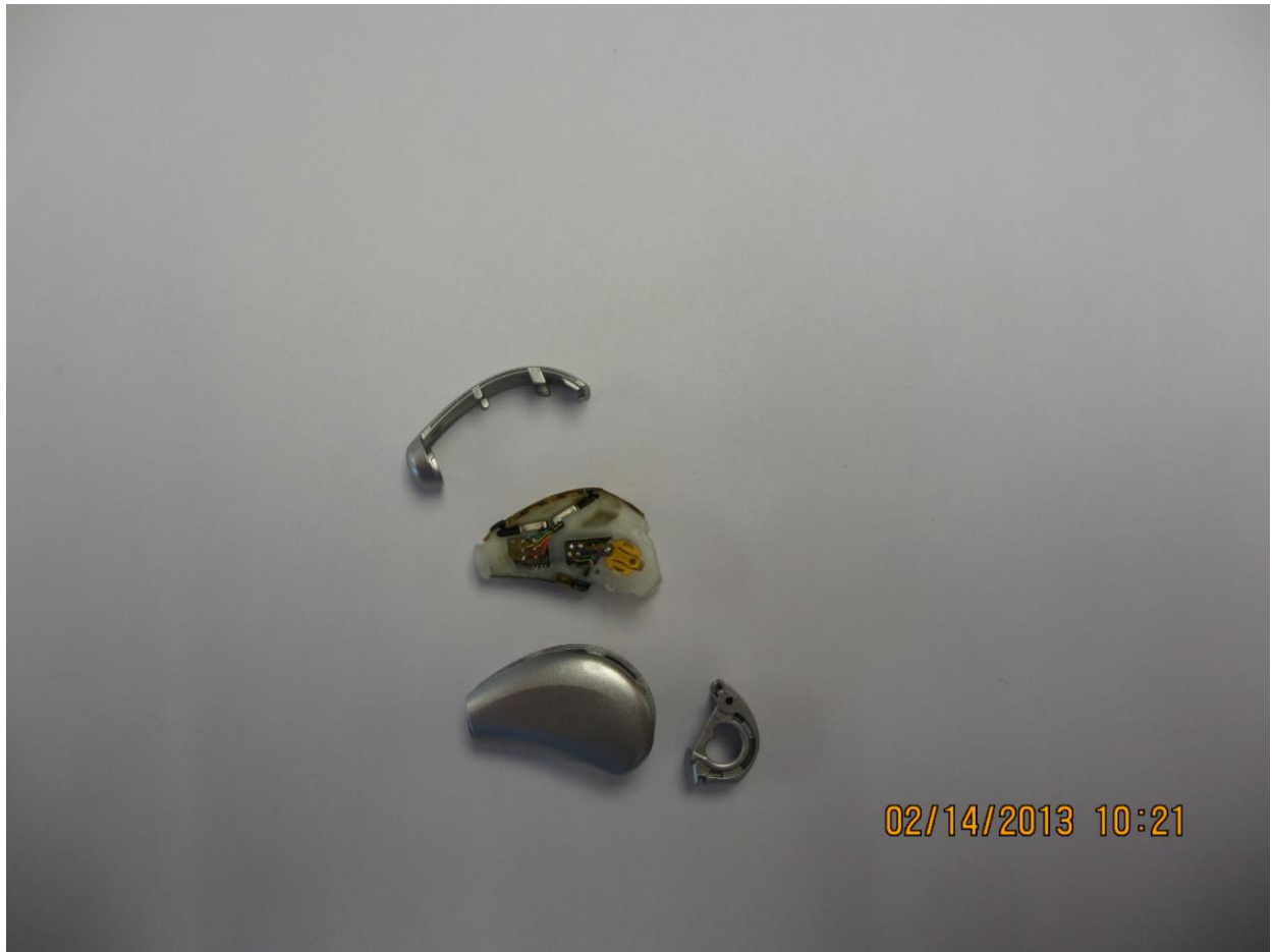
XF13 Internal Photo showing spine assembly removed from case
