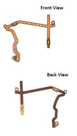
Figure 1 2.4 GHz Antenna
