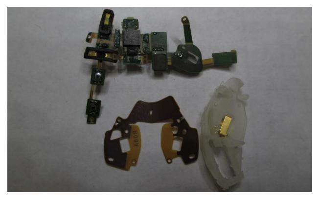
Unfolded flex circuit and 2.4 GHz antenna, bottom view
